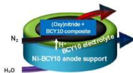
Figure 1. Schematic electrochemical NH 3 production using a PCEC.
