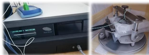
Figure 2. Thermal constant measuring device: Hot Disk TPS 500 and Pico Data Logger (left) and samples (right)
