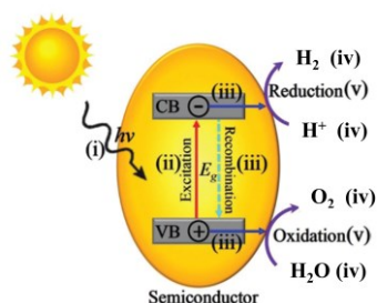
Figure 1. The mechanism of photocatalytic water splitting on the semiconductor-based photocatalyst [1].
